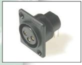
ACF / PC 3 Pin right angle PCB mounting Female XLR with counter sunk mounting holes for M3 screw fixing. XACF / PC has non counter sunk mounting holes for self-tap screw fixing. Nickel Silver plated Brass contacts.
