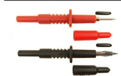
**TPR/1S** Spiked test probe. Unfused. Has 4mm. shrouded socket connection, so converts 4mm. shrouded plug into a test prod lead. 1KV CAT III with tip cover fitted, CAT II without.
