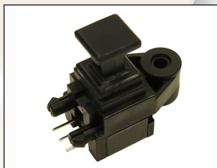
OTJ-1/ORJ-1 Single Optical Transmitter and Receiver Jack. Right angle PCB mount with self tapping hole for panel mounting. Removable plug-in cover.
