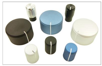
Knobs for professional equipment - comprising machined aluminium shell on moulded plastic inner. Push on fixing. Max shaft depth 11mm.
