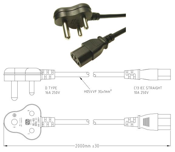
This power cord has an Indian 3 pin D type mains plug on one end and an IEC C13 type connector on the other end. The power lead features integrated strain reliefs that provide additional protection and support to the connectors. Conforms to BIS IS1293 + IS694
